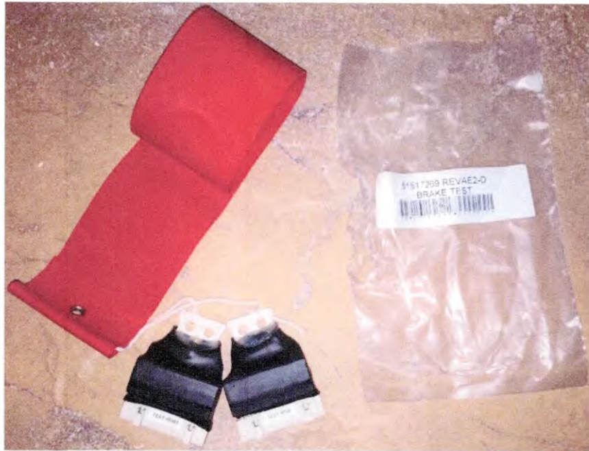
Test Plugs to Lift Brakes Individually for Performing 125% Load Test
