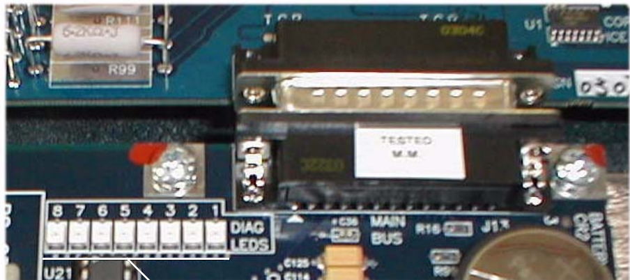
Figure 3.3 iLink CTP Board Diagnostic LEDs
