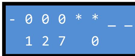
Press the up arrow to change the 0 to a 1 and then press enter. The error has now been reset. Return to the main diagnostic display by pressing escape several times.
