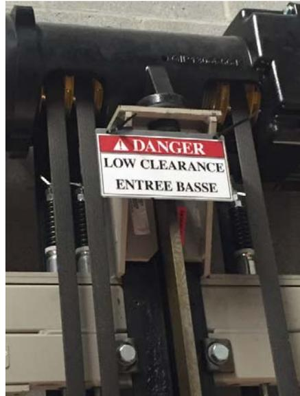
4 & 3 Belt Installations with Neoprene Belts (on left) and Older Rubber Belts (on right)
