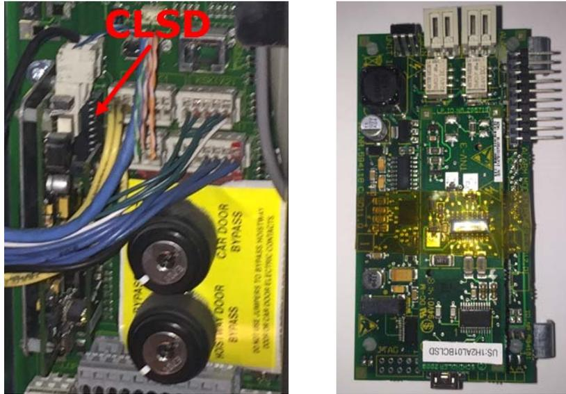
To remove the CLSD board, remove power to the controller by opening the disconnect or opening the JHS breaker in the control panel.
