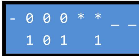
Press the enter button again and the 101 reset will be performed. Press the escape button (first button on the left) several times to get back to the main screen.
