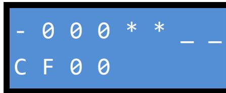
This screen lets you know that you are in the configuration menu and at configuration parameter 00 (CF00). If you press the up button CF00 will change to CF01, CF02, etc. to scroll through the various configuration parameters.
