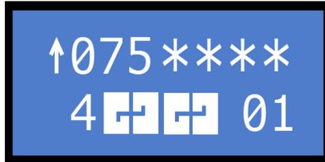
In the upper row of the diagnostic screen, the arrow indicates that the elevator is currently moving in the up direction. If it were moving in the down direction a down arrow would be present. When the car is stopped a minus sign (-) is displayed.
